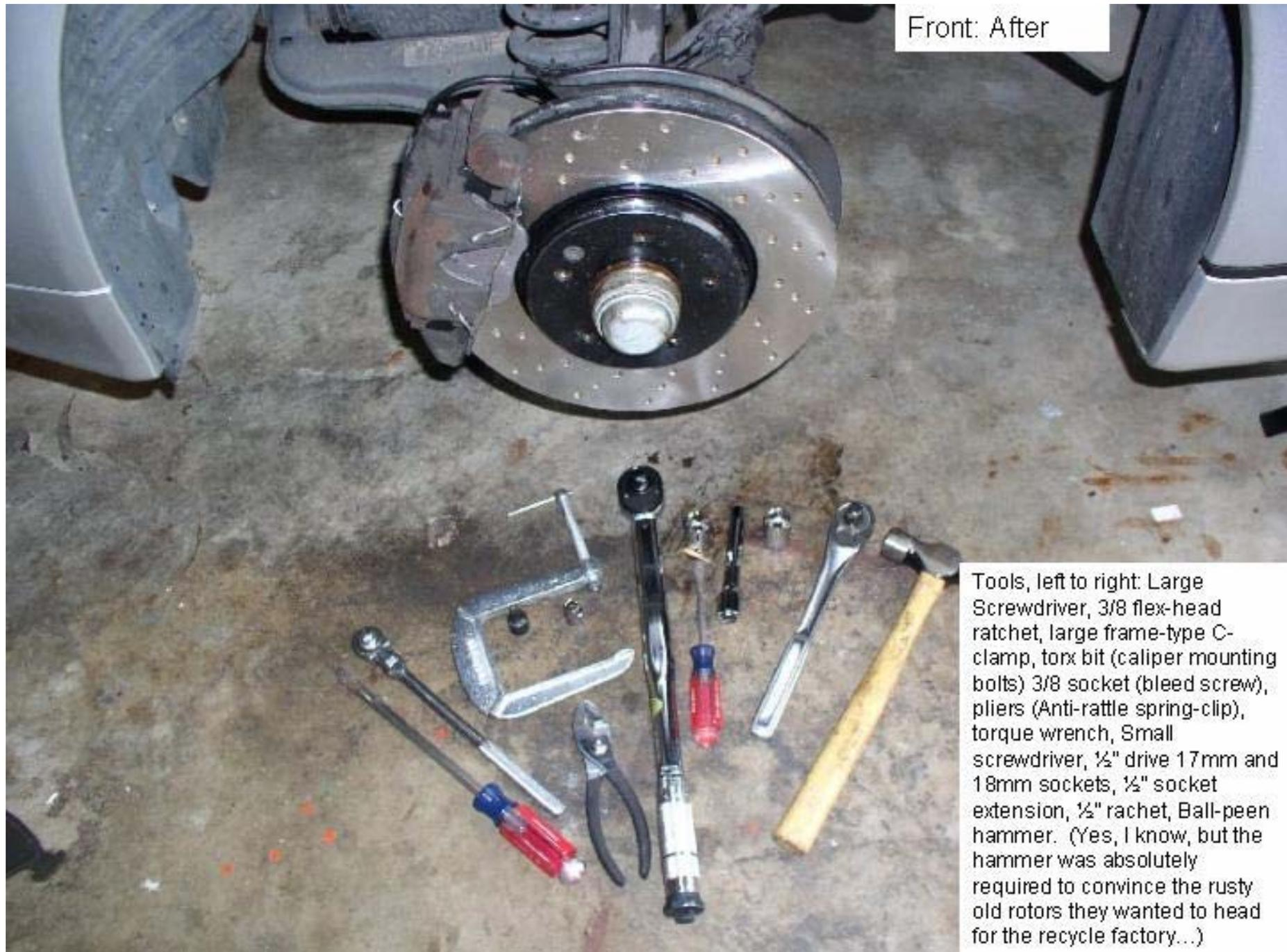
Tools, left to right: Large Screwdriver, 3/8 flex-head ratchet, large frame-type C-clamp, torx bit (caliper mounting bolts) 3/8 socket (bleed screw), pliers (Anti-rattle spring-clip), torque wrench, Small screwdriver, 1/2" drive 17mm and 18mm sockets, 1/2" socket extension, 1/2" ratchet, Ball-peen hammer. (Yes, I know, but the hammer was absolutely required to convince the rusty old rotors they wanted to head for the recycle factory...)
